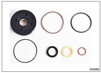
**IMPORTANT:** Use of Trim & Tilt Piston Seal Tool Kit 5008918 and Spanner Tool 352932 are required to install the components of these kits.
