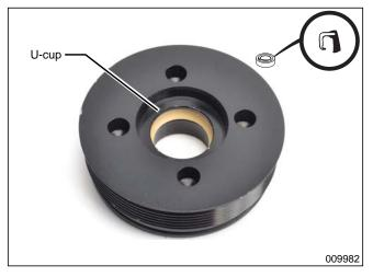
Lubricate and install the new wiper seal with the lip side facing the top of the end cap.
