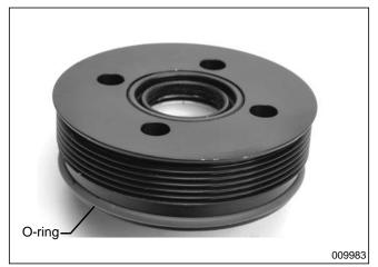
Lubricate the threads of the end cap prior to assembly.
