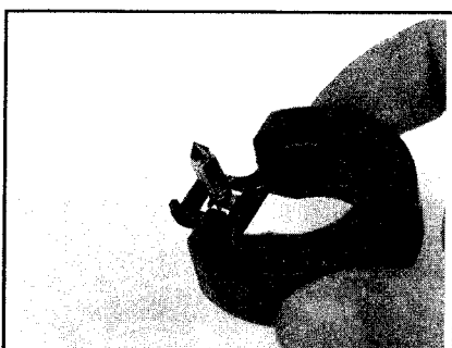
Fig. 42 Thoroughly inspect the float and float needle for damage . . .
