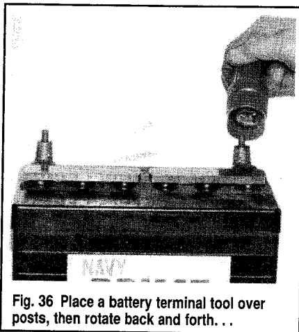
Fig. 37 . . .until the internal brushes expose a fresh, clean surface on the post
