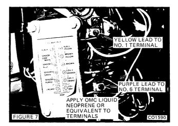
7. Connect terminal end of purple lead to number 6 terminal with one existing solid purple lead. See Figure 7.
