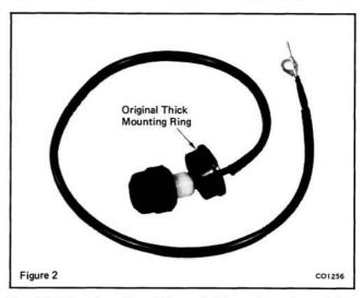
On 1977 and earlier 9.9 and 15 outboard models, you will use the original mounting bushing plus the mounting ring furnished in the kit as shown in Figure 3.
