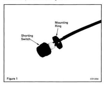
On 6 through 50 rope start outboard models with the exception of the 9.9 and 15, use switch and mounting ring furnished in kit. On 1978 9.9 and 15 outboard models, discard mounting ring from this kit. Use original plastic ring on engine with new switch as shown in Fig. 2.
