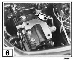
4 Apply *Triple-Guard®* grease to post **(a)**. Install cam follower on post, and install O-ring on post, in groove.
