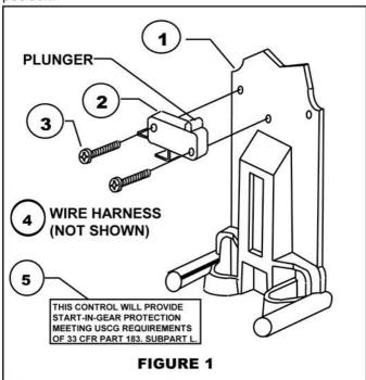
Route the wires so they will not in any way come in contact with the cable or moving parts of the control. If necessary, the switch can be mounted on the right side (left side mounting shown in Figure 1). Connect one wire of the switch to the "Start" terminal on the ignition switch and the other to the **positive** terminal of the starter solenoid (see Figure 2 and warning).
